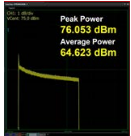
▲ Fig. 7 Uncorrected 40 kW pulse.
